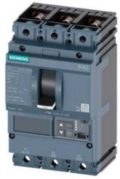
CIRCUIT BREAKER 3VA2 IEC FRAME 160 BREAKING CAPACITY CLASS L ICU=150KA @ 415 V 3POLE, LINE PROTECTION ETU550, LSI, IN=63A OVERLOAD PROTECTION IR=25A ...63A SHORT CIRCUIT PROTECTION ISD=0,6..10X IN, II=1,5..12X IN NEUTRAL PROTECTION OPTIONAL WITH EXT. CT,UPTO 160% BUSBAR CONNECTION
