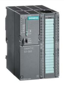
SIMATIC S7-300, CPU 313C-2 PTP COMPACT CPU WITH MPI, 16 DI/16 DO, 3 FAST COUNTERS (30 KHZ), INTEGRATED INTERFACE RS485, INTEGRATED 24V DC POWER SUPPLY, 128 KBYTE WORKING MEMORY, FRONT CONNECTOR (1 X 40PIN) AND MICRO MEMORY CARD REQUIRED
