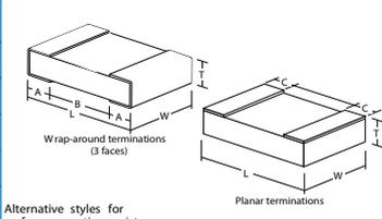
Alternative styles for surface mounting resistors
