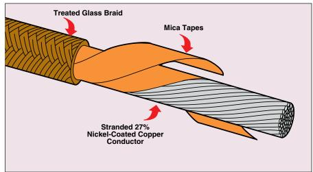
HTMG high-temperature lead wires are designed for appliances and industrial heating products—such as commercial food service equipment, heaters, heat treating furnaces, kilns, heater elements and other applications up to 450°C (842°F).
