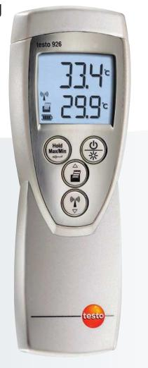
The testo 926 is an exact temperature measuring instrument which is particularly suited to applications in the food sector. In addition to the broad selection of classical probes with a cable, a wireless radio probe can also be connected if required. The dishwasher-safe TopSafe protects the instrument from dirt, water and impact.
