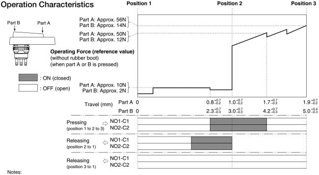
• When rubber boot is used, operating force depends on the operating temperature.
