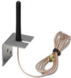
Omnidirectional antenna, 2.4 GHz, 2 dBi, linear vertical, 1.5 m cable, RSMA (male), IP65, 50 Ω impedance
