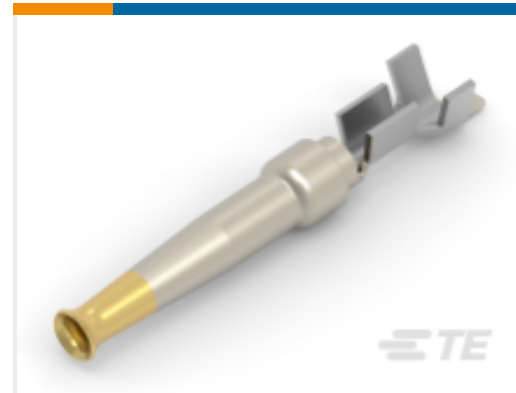
TE Part #1658537-1 D-Sub Conn Contacts: Socket, Phosphor Bronze, Signal, Size 20
