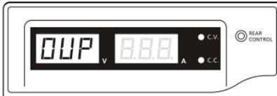
To reset the warning, switch off the unit and remove all loading. Switch the unit back on again and it should resume normal operation. If this problem persists, please contact and consult with your agent.
