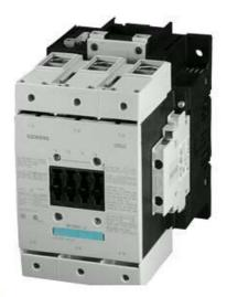
CONTACTOR, 55KW/400V/AC-3 AC(40...60HZ)/DC OPERATION UC 200...277V AUXIL. CONTACTS 2NO+2NC 3-POLE, SIZE S6 WITH BOX TERMINALS ELECTRONIC OPERATING MECHANISM WITH PLC INTERFACE 24V DC SCREW TERMINAL
