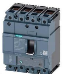
CIRCUIT BREAKER 3VA1 IEC FRAME 160 BREAKING CAPACITY CLASS S ICU=36KA @ 415 V 4-POLE, LINE PROTECTION TM240, ATAM, IN=50A OVERLOAD PROTECTION IR=35A ...50A SHORT CIRCUIT PROTECTION II=5...10 X IN NEUTRAL PROTECTION 100% CABLE CONNECTION
