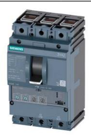
CIRCUIT BREAKER 3VA2 IEC FRAME 100 BREAKING CAPACITY CLASS M ICU=55KA @ 415 V 3POLE, LINE PROTECTION ETU330, LIG, IN=40A OVERLOAD PROTECTION IR=16A ...40A SHORT CIRCUIT PROTECTION II=1,5...12 X IN GROUNDFAULTPROTECTION IG=0,2... 1 X IN, TG=0,1/0,3MS CABLE CONNECTION
