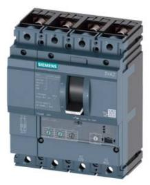
CIRCUIT BREAKER 3VA2 IEC FRAME 160 BREAKING CAPACITY CLASS L ICU=150KA @ 415 V 4POLE, LINE PROTECTION ETU320, LI, IN=25A OVERLOAD PROTECTION IR=10A ...25A SHORT CIRCUIT PROTECTION II=12 X IN NEUTRAL PROTECTION ADJUSTABLE(OFF,100%) BUSBAR CONNECTION
