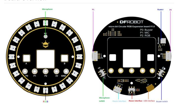
Note: After uploading the micro: bit program you need to connect the USB cable to the expansion board for power, You can also use 3.5-5.0 V power supply to power from the expansion board battery!
