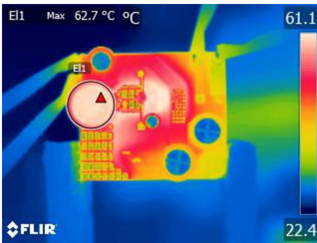
Figure 12 – Buck Choke (EI1), 62.7 °C. 85 VAC, 800 mA Output.
