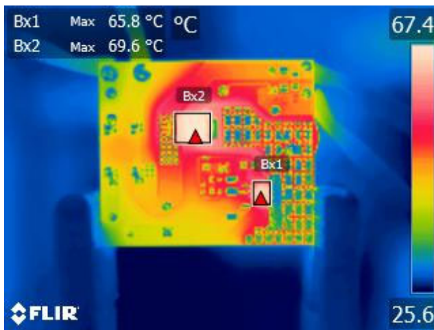
Figure 14 – LNK3209D (Bx1), 65.8 °C. Buck Diode (Bx2), 69.6 °C. 85 VAC, 800 mA Output.
