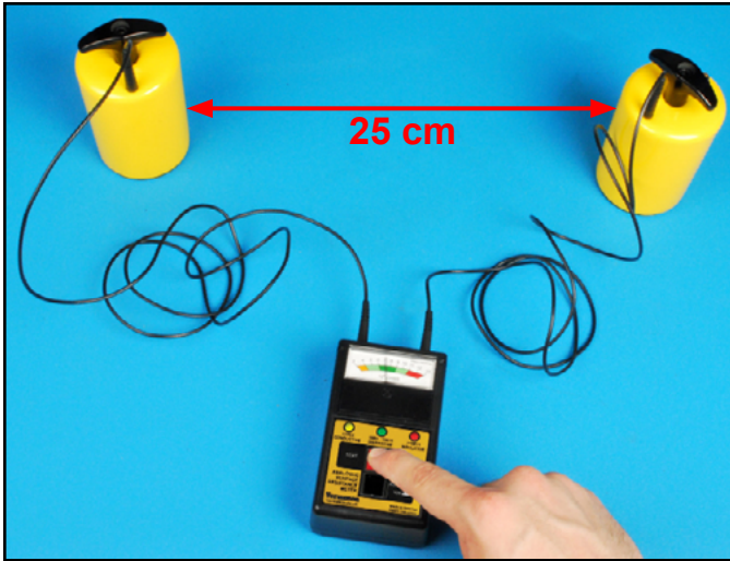
Figure 4. Using the test leads and two 2.27 kg electrodes to measure R_{p-p} of worksurfaces (place electrodes 1 m apart for flooring)
