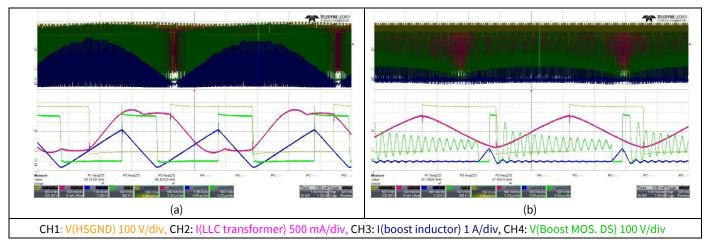
Figure 18 Boost and LLC waveforms at 120  $V_{RMS}$  (a)  $V_{dim} = 10 V$ ,  $V_{LED} = 76 V$  and (b)  $V_{dim} = 0.1 V$ ,  $V_{LED} = 65 V$
