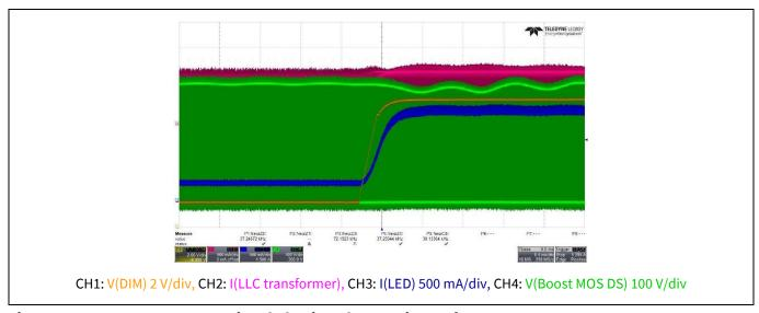
Figure 21 LED current transient behavior when V<sub>dim</sub> jumps from 0.1 V to 10 V
