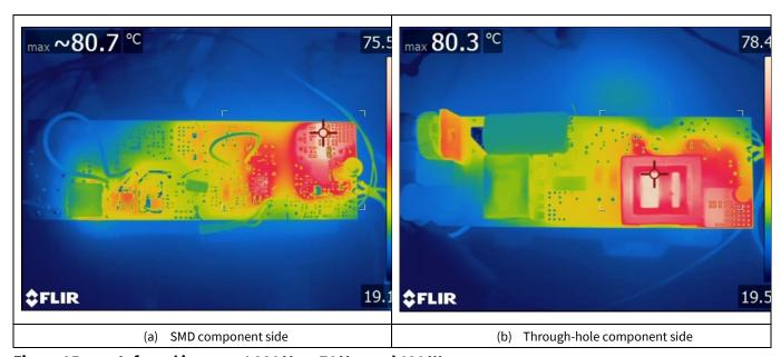
Figure 25 Infrared images at 230 V<sub>RMS</sub>, 76 V<sub>LED</sub> and 130 W
