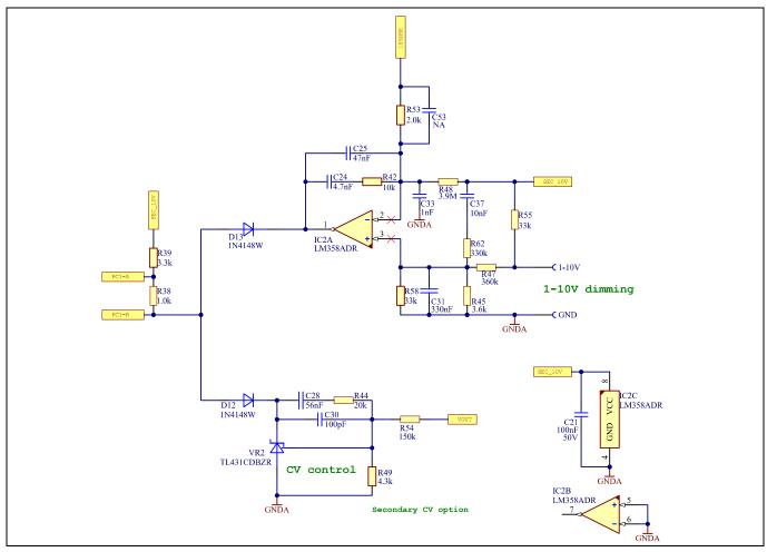
Figure 5 Schematic of the secondary-side control circuit
