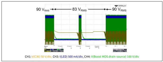
Figure 22 Brown-out protection (brown-out point at 83 V<sub>RMS</sub>)
