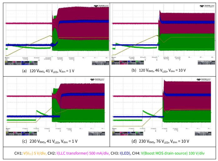
Figure 20 Start-up behavior of the V<sub>cc</sub>, LED current, LLC transformer current at different operating conditions (a to d)
