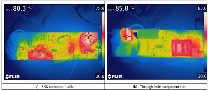
Figure 24 Infrared images at 120 V<sub>RMS</sub>, 76 V LED and 130 W
