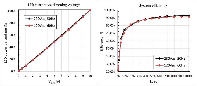
Figure 10 LED current vs. dimming voltage (V<sub>LED</sub> = 76 V)
