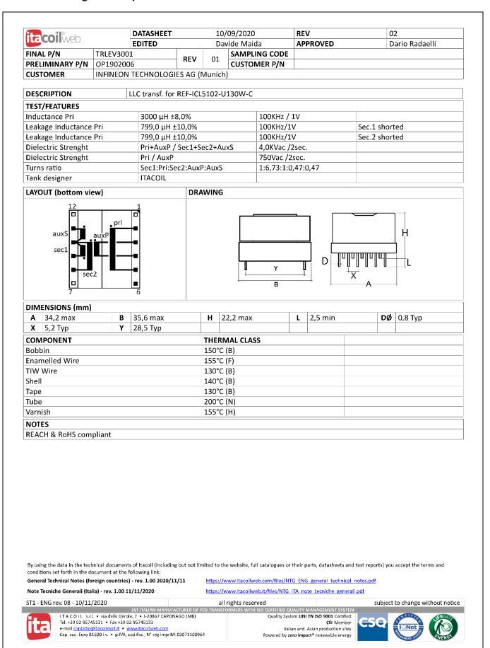
Figure 30 Integrated LLC transformer - TR1
