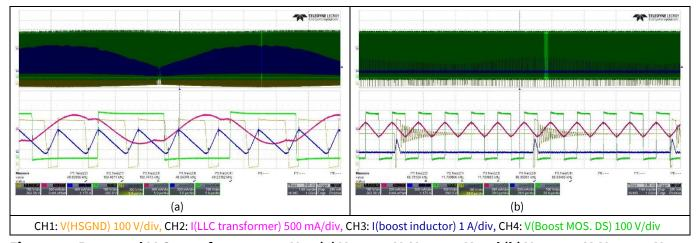
Figure 17 Boost and LLC waveforms at 230  $V_{RMS}$  (a)  $V_{dim} = 10 V$ ,  $V_{LED} = 46 V$  and (b)  $V_{dim} = 0.1 V$ ,  $V_{LED} = 39 V$
