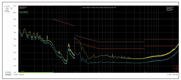
Figure 26 Conducted EMI at 230  $V_{\text{RMS}}$  input and 130 W output
