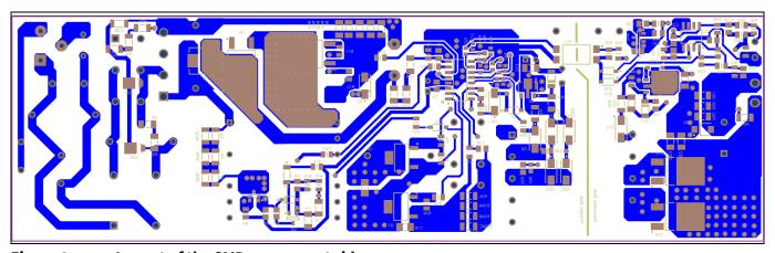
Figure 8 Layout of the SMD component side
