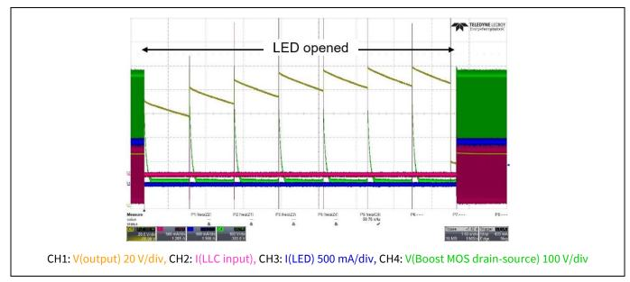
Figure 23 LED open protection
