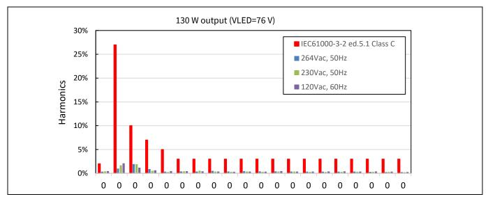
Figure 14 Input current harmonics at 130 W load
