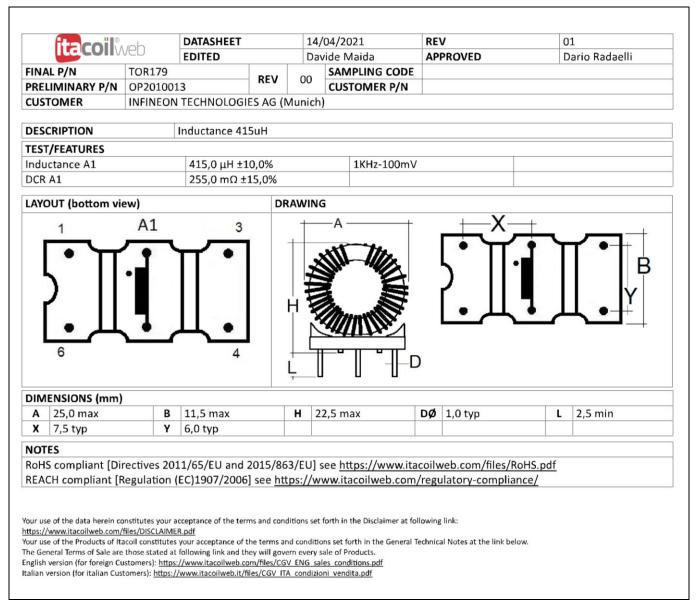
Figure 28 Differential mode EMI choke - L1
