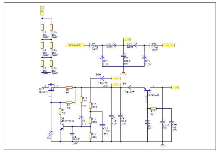
Schematic of the start-up and Vcc circuit Figure 4
