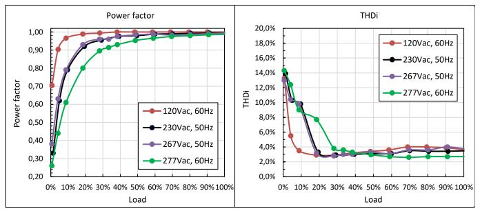
Figure 12 Power factor vs. load
