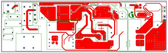
Figure 7 Layout of the through-hole component side
