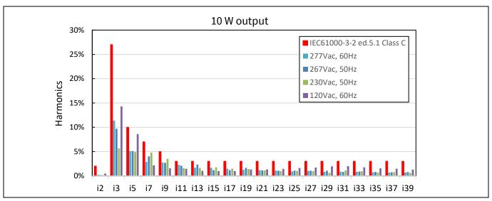
Figure 15 Input current harmonics at 10 W load
