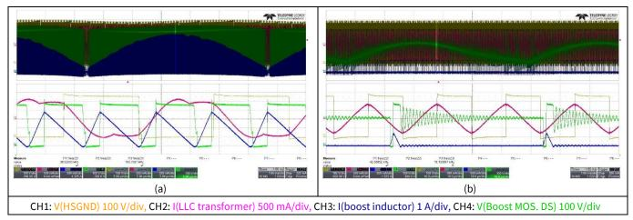
Figure 16 Boost and LLC waveforms at 230  $V_{RMS}$  (a)  $V_{dim} = 10 V$ ,  $V_{LED} = 76 V$  and (b)  $V_{dim} = 0.1 V$ ,  $V_{LED} = 65 V$
