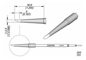
This cartridge has a 30 mm long tip which allows you to solder hard-to-access applications.
