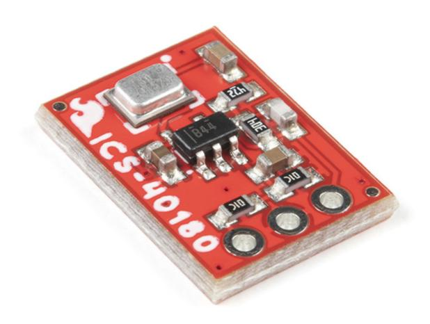
The SparkFun Analog MEMS Microphone Breakout makes it easy to work with the InvenSense ICS-40180 analog microphone. This board features an OpAmp to bring the output of the microphone to a usable level, allowing you to plug directly into an ADC on a microcontroller or something like the <u>SparkFun Spectrum Shield</u>.
