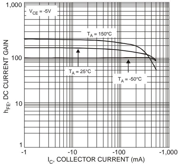
Fig. 1 Typical DC Current Gain vs. Collector Current
