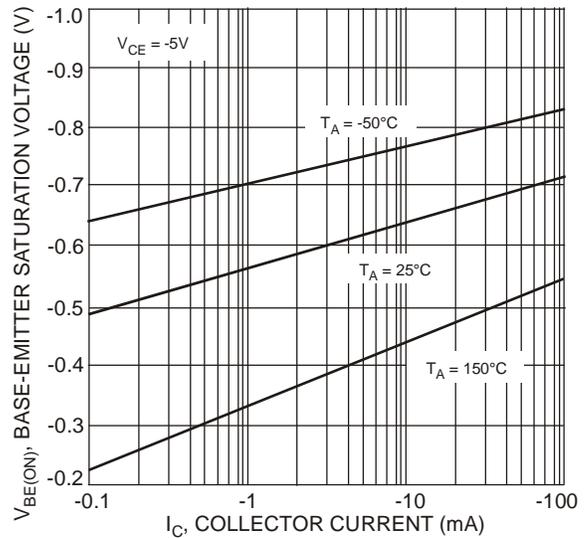
Fig. 2 Typical Base-Emitter Saturation Voltage vs. Collector Current
