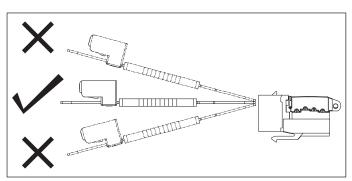
Key must be inserted perpendicular to the socket
