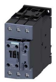
CONTACTOR,AC3:22KW/400V, 1NC+1NO,200VAC50HZ/200.220V60HZ 3-POLE, SIZE S2, SCREW TERMINAL
