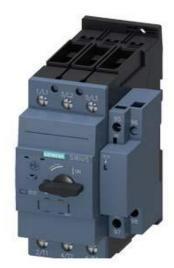
CIRCUIT BREAKER, SIZE S2, FOR MOTOR PROTECTION, CLASS 10, W. OVERLOAD RELAY FUNCTION A-RELEASE 9.5...14A, N-RELEASE 208A, STANDARD BREAKING CAPACITY
