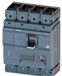
CIRCUIT BREAKER 3VA2 IEC FRAME 630 BREAKING CAPACITY CLASS H ICU=85KA @ 415 V 4-POLE, LINE PROTECTION ETU850, LSI, IN=500A OVERLOAD PROTECTION IR=200A ...500A SHORT CIRCUIT PROTECTION ISD=0,6..10X IN, II=1,5..14X IN NEUTRAL PROTECTION ADJUSTABLE (OFF, UPTO 100%) BUSBAR CONNECTION
