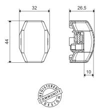
Floor surface water sensor for connection to electrode terminals (B1 and B3) of 72.01 or 72.11 level control relay, set in Emptying function (ES or E respectively).
