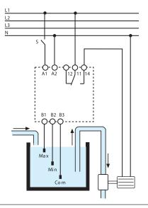
The 72 series level control relays work by measuring the resistance through the liquid, between the common (B3) electrode and Min. and Max. electrodes (B2 and B1). If the tank is metalic, then this can be substituted as the B3 electrode.
