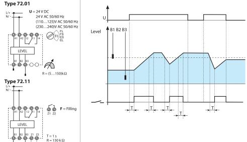
Filling Control – between Min. and Max. levels.
