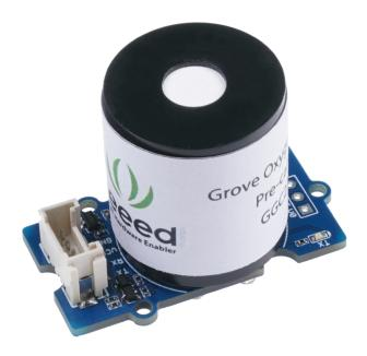
Grove - Oxygen Sensor Pro(GGC2330-O2) is a kind of sensor to test the oxygen concentration in air, which is based on the principle of the electrochemical cell to the original work. When it starts to work, it will produce a current proportional to the concentration of oxygen, then you can determine the concentration of oxygen by measuring the Current size.
