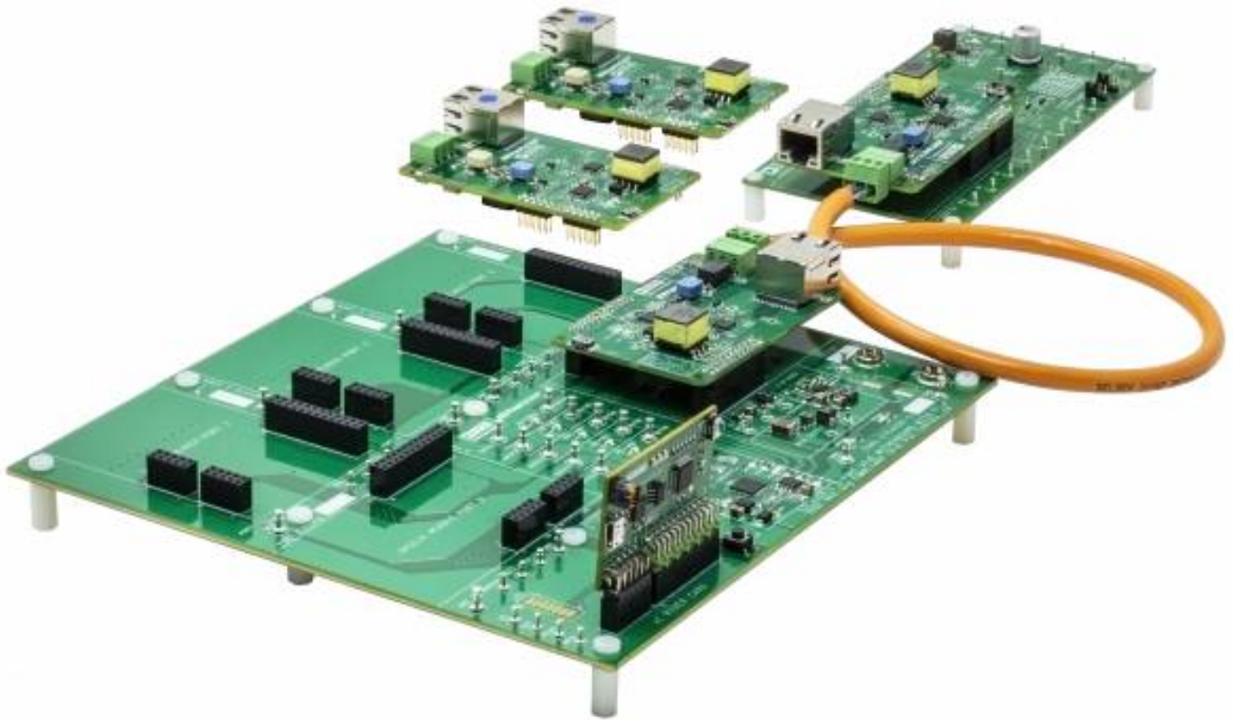
Figure 2. EVAL-SPoE-KIT-AZ 802.3cg SPoE Class 10 through 15 and 10BASE-T1L SPE evaluation kit.
