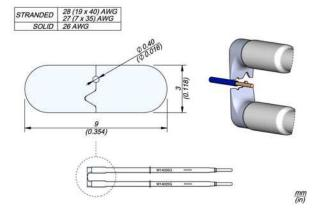
W14026G is specially designed for stripping high-temperature wire insulations made of thermostable materials such as Teflon\*, Kapton\*, silicone rubber, etc, of 26 AWG (0.40 mm / 0.0157 in).
