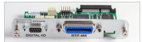
KTTI-GPIB GPIB interface with 6 digital I/O ports.
