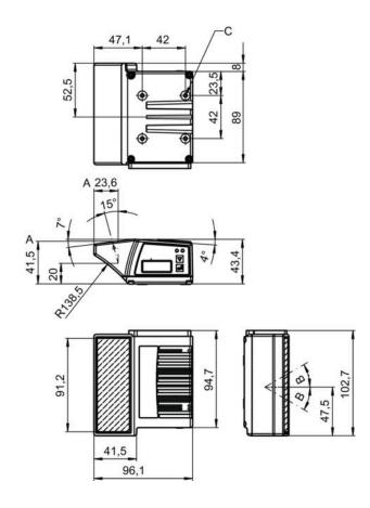
A Optical axis B Deflection angle of the laser beam:  $\pm$  30  $^{\circ}$  C M4 thread (5 deep)
