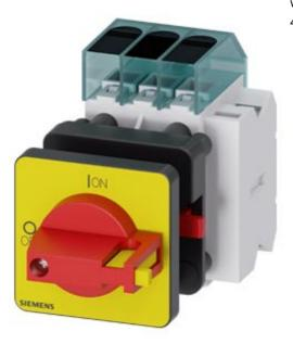
Switch disconnector 3LD3, main switch 3-polig, lu 63A operational switch at AC-23 A at 400 V 22,0 kW front mounted Base mounting with center-hole 22,5 mm knob-operated mechanism red/yellow 48 x 48 mm with auxiliary 1NO+1NC
