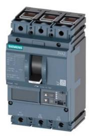
CIRCUIT BREAKER 3VA2 IEC FRAME 160 BREAKING CAPACITY CLASS H ICU=85KA @ 415 V 3POLE, LINE PROTECTION ETU550, LSI, IN=63A OVERLOAD PROTECTION IR=25A ...63A SHORT CIRCUIT PROTECTION ISD=0,6..10X IN, II=1,5..12X IN NEUTRAL PROTECTION OPTIONAL WITH EXT. CT,UPTO 160% CABLE CONNECTION
