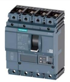
CIRCUIT BREAKER 3VA2 IEC FRAME 250 BREAKING CAPACITY CLASS M ICU=55KA @ 415 V 4POLE, LINE PROTECTION ETU560, LSIG, IN=160A OVERLOAD PROTECTION IR=64A ...160A SHORT CIRCUIT PROTECTION ISD=0,6..10X IN, II=1,5..12X IN NEUTRAL PROTECTION ADJUSTABLE (OFF, UPTO 160%) GROUNDFAULT, SWITCHABLE IG=0,2... 1 X IN, TG=0,050,8MS BUSBAR CONNECTION
