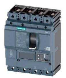
CIRCUIT BREAKER 3VA2 IEC FRAME 250 BREAKING CAPACITY CLASS M ICU=55KA @ 415 V 4POLE, LINE PROTECTION ETU850, LSI, IN=250A OVERLOAD PROTECTION IR=100A ...250A SHORT CIRCUIT PROTECTION ISD=0,6..10X IN, II=1,5..10X IN NEUTRAL PROTECTION ADJUSTABLE (OFF, UPTO 100%) BUSBAR CONNECTION
