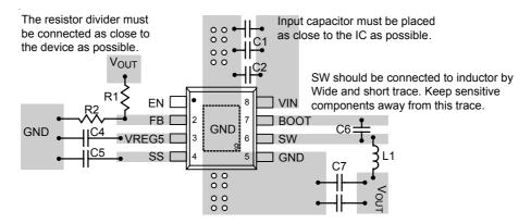
Figure 7. PCB Layout Guide for SOP-8 (Exposed Pad) Package
