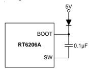
Figure 5. External Bootstrap Diode
