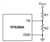
Figure 4. Output Voltage Setting
