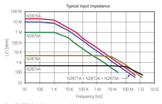
Figure 10. N2870A Series input impedance vs. frequency characteristics.
