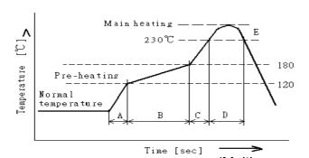
Slope of temp. rise 1 to 5 °C/sec 50 to 150 Heat time sec В 120 to 180 Heat temperature  $^{\circ}$ C 1 to 5  $\mathbf{C}$ Slope of temp. rise °C/sec 90~120 D Time over 230°C sec Peak temperature 255~260  $^{\circ}$ C Е Peak hold time 10 max. sec 3 No. of mounting times
