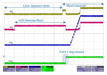
Figure 11: LED1 is shorted-to-GND initially, then released. After the fault is removed, the IC auto-recovers and proceeds with soft-start. FAULT is released at the end of LED detection phase.
