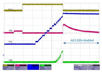
Figure 42: A80601-1 startup with LED2 string open.  $V_{\rm OUT}$  hits OVP and all LED string are disabled. FAULT pin goes Low and IC remains latched off until reset.
