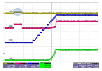
Figure 10: Normal startup showing LED1 channel is disabled with a 2.37 k $\Omega$  resistor to GND. Total LED current = 100 mA × 3.
