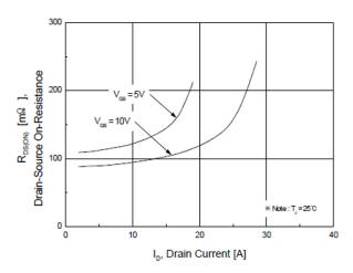
Figure 51: Chart showing On-Resistance varies with Darin Current and Gate Voltage.
