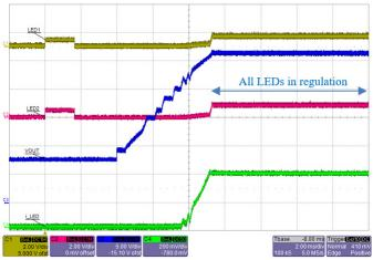
Figure 38: A80601 Normal startup sequence showing voltage at LED1 and LED2 pins.  $V_{IN}$  = 6 V, output = 8 × WLED in series, current = 4 × 100 mA
