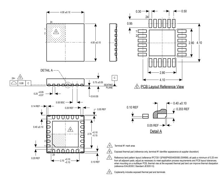
Figure 49: Package ES, 24-Pin 4 mm × 4 mm QFN with Exposed Thermal Pad and Wettable Flank
