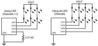
Figure 8: How to signal an unused LED channel during startup LED detection phase
