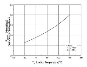
Figure 52: Nominalized On-Resistance vs. Junction Temperature at  $V_{GS}$  = 10 V. Note that resistance increases by 100% when temperature rises from 25°C to 150°C.
