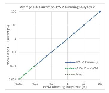
Figure 30: How to achieve 100,000:1 dimming ratio by using both PWM and APWM. Test conditions:  $V_{IN}$  = 12 V,  $V_{OUT}$  = 25 V (8 × WLED), total LED current = 400 mA, PWM frequency = 200 Hz, APWM frequency = 100 kHz.
