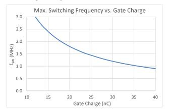
Figure 53: Maximum Switching Frequency vs. Gate Charge (to keep average  $V_{DRV}$  current under 36 mA).
