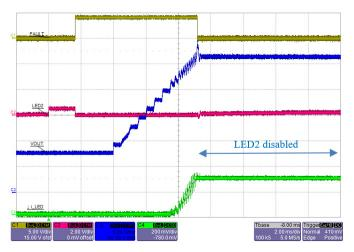
Figure 41: A80601 startup with LED2 string open.  $V_{OUT}$  hits OVP at ~28 V and LED2 is removed from regulation. FAULT pin goes Low but remaining LED strings continue to operate.
