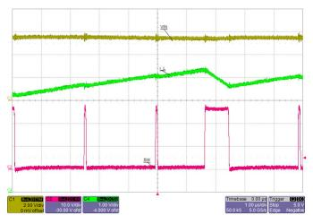
Figure 46: When peak current through the inductor reaches  $\sim$ 5.4 A, overcurrent protection kicks in to truncate the present switching cycle.
