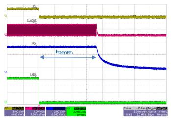
Figure 34: After EN = L for  $\sim$ 16 ms, the IC completely shuts down so VDD (Blue) decays.
