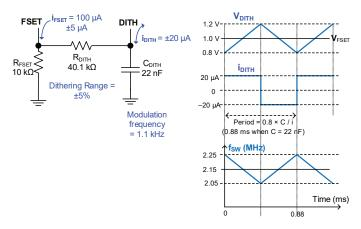
Figure 17: How to Program Switching Frequency Dithering Range and Modulation Frequency There are no hard limits on dithering range and modulation frequency. As a general guideline, pick a dithering range between  $\pm 5\%$  and 10%, with the modulation frequency between 1 kHz and 3 kHz. In practice, using a larger dithering range and/or higher modulation frequency do not generate any noticeable benefits.
