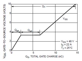
Figure 54: Gate Charge vs. Gate-Source Voltage chart for a suitable MOSFET (NVD5867NL). Note that its plateau is at ~3.5 V, and its total gate charge is about 10 nC as  $V_{GS}$  ramps up from 0 to 6.5 V.
