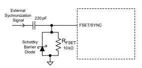
Figure 16: Countermeasure for External Sync Stuck-at-Low Fault
