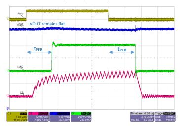
Figure 24: A80601 PWM dimming operation with PEB delay set to 3  $\mu s.$  Note that  $V_{OUT}$  ripple is reduced to ~0.2 V.
