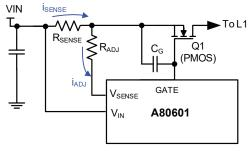
$V_{\text{IN}} - V_{\text{SENSE}} = R_{\text{SC}} \times i_{\text{SENSE}} + R_{\text{ADJ}} \times i_{\text{ADJ}}$
