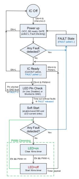
Figure 36: Simplified A80601 Startup Flowchart
