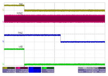
Figure 35: As long as EN = H, the IC does not shut down VDD and CLKOUT. But internal latched faults are cleared by PWM = L for  $\sim$ 16 ms.
