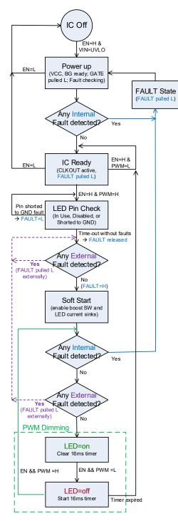
Figure 37: Simplified startup flow chart for A80601-1, showing responses to both Internal and External FAULT signals
