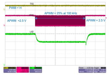
Figure 28: PWM = H. Total LED current drops from 400 mA (4  $\times$  100 mA/ch) to 300 mA when APWM of 25% duty cycle is applied. Note that LED current takes ~0.5 ms to settle after change in APWM.
