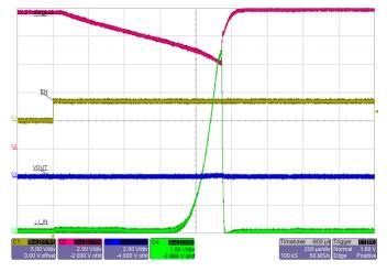
Figure 48: Startup into an output shorted-to-GND fault. Input OCP is tripped when current (Green trace) exceeds ~6.5 A. PMOS Gate (Red) is turned off immediately and IC latches off.
