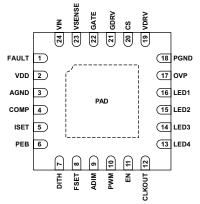
Package ES, 24-Pin QFN Pinouts
