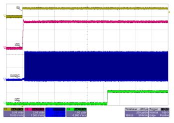
Figure 6: Startup showing EN, VDD, CLKOUT, and ISET (PWM = L). Note that CLKOUT is available as soon as  $V_{DD}$  ramps up, even though Boost stage and LED drivers are not yet enabled.
