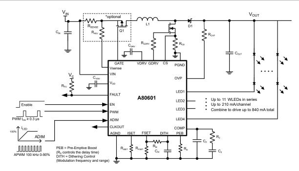
Figure 1: A80601 in Boost configuration where  $V_{OUT}$  is higher than  $V_{IN}$
