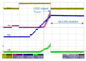
Figure 40: A80601-1 startup sequence when LED string#2 has a partial-short fault (6 × WLED instead of 8). As soon as LED2 pin rises above  $V_{LEDSD}$  (~5 V), the channel is disabled but FAULT remains High.
