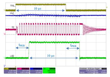
Figure 21: Zoom in view for PWM on-time = 10  $\mu$ s. Notice that the LED current is shifted with respect to PWM signal. Ripple at V<sub>OUT</sub> is ~0.2 V when using 2 × 4.7  $\mu$ F MLCC as output capacitors.
