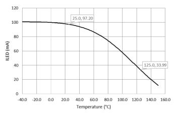
Figure 33: LED current varies with temperature when using thermistor NTCS0805E3684JXT for thermal foldback
