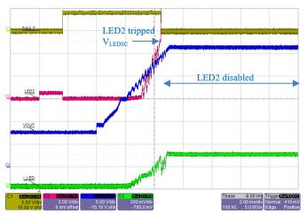
Figure 39: A80601 startup sequence when LED string#2 has a partialshort fault (6 × WLED instead of 8). As soon as LED2 pin rises above  $V_{LEDSC}$  (~5 V), the channel is disabled and FAULT = Low.
