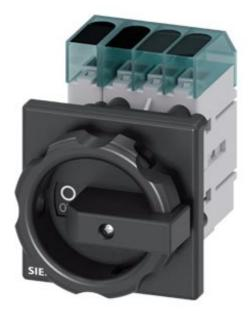
Switch disconnector 3LD3, main switch 3-polig + N, lu 32A operational switch at AC-23 A at 400 V 11,5 kW front mounted Base mounting with center-hole 22,5 mm rotary operationg mechanism black 66 x66 mm
