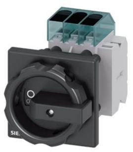
Switch disconnector 3LD3, main switch 3-polig, lu 63A operational switch at AC-23 A at 400 V 22,0 kW front mounted Base mounting with center-hole 22,5 mm knob-operated mechanism black 66 x66 mm with auxiliary 1NO+1NC
