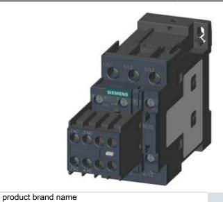
CONTACTOR, AC-3, 7.5KW/400V, 2NO+2NC, DC 110V, 3-POLE, SZ S0 SCREW TERMINAL REMOVABLE AUX. SWITCH
