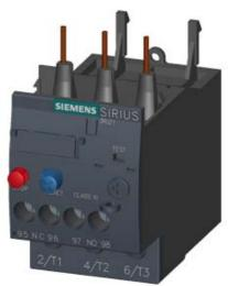
OVERLOAD RELAY 7.0...10 A FOR MOTOR PROTECTION SZ S0, CLASS 10, F. MOUNTING ONTO CONTACTOR MAIN CIRCUIT: SCREW TERMINAL AUX. CIRCUIT: SCREW TERMINAL MANUAL-AUTOMATIC-RESET
