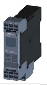
DIGITAL MONITORING RELAY CURRENT MONITORING, 22.5MM FOR IO-LINK 0.05 TO 10.0A AC/DC OVER- AND UNDERCURRENT CONVERTER SCALING FACTOR HYSTERESIS 0.01 TO 5.0A ON DELAY TIME TRIPPING DELAY TIME 1 CHANGE-OVER CONTACT, SPRING-LOADED TERMINAL
