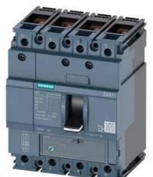
CIRCUIT BREAKER 3VA1 IEC FRAME 160 BREAKING CAPACITY CLASS N ICU=25KA @ 415 V 4-POLE, LINE PROTECTION TM220, ATFM, IN=20A OVERLOAD PROTECTION IR=14A ...20A SHORT CIRCUIT PROTECTION II=10 X IN NEUTRAL UNPROTECTED BUSBAR CONNECTION
