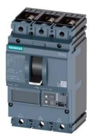
CIRCUIT BREAKER 3VA2 IEC FRAME 250 BREAKING CAPACITY CLASS L ICU=150KA @ 415 V 3POLE, LINE PROTECTION ETU550, LSI, IN=160A OVERLOAD PROTECTION IR=64A ...160A SHORT CIRCUIT PROTECTION ISD=0,6..10X IN, II=1,5..12X IN NEUTRAL PROTECTION OPTIONAL WITH EXT. CT,UPTO 160% BUSBAR CONNECTION
