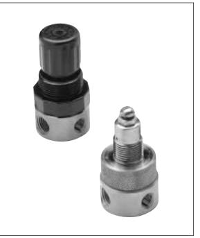
Ordering Information. Models listed include PTF threads, plastic bonnet with knob adjustment, non-relieving diaphragm, 5 to 100 psig (0.3 to 7 bar) outlet pressure adjustment range†, and without gauge.
