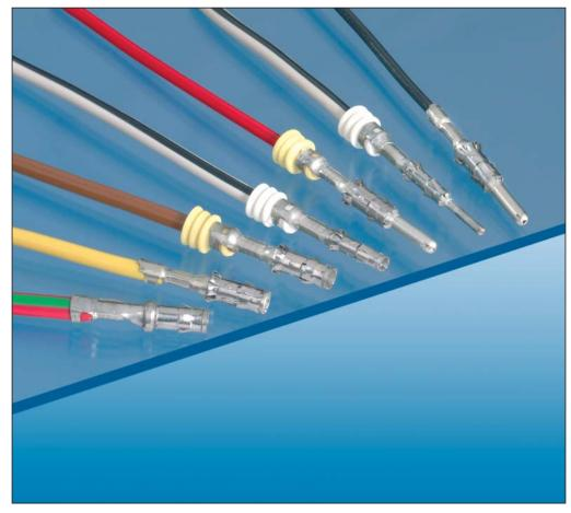
The diameter 1.5 mm and diameter 2.5 mm round contact systems developed by Tyco Electronics is mainly used in the automotive industry. Due to its wide range of performance possibilities, this contact system is in use in the engine compartment for aggregate or sensor connections.
