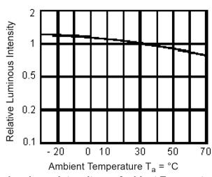
Luminous Intensity vs. Ambient Temperature
