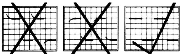
And adjust the trimmer located in the BNC connector for a flat-topped square wave.
