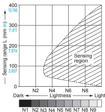
The sensing region (typical) is represented by oblique lines in the left figure. However, the sensitivity should be set with an enough margin because of slight variation in products.
